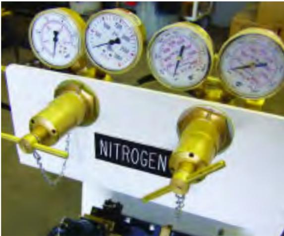
3-bottle Lo-Hi Nitrogen regulator mounted on 3-bottle tilting cart with nitrogen booster
