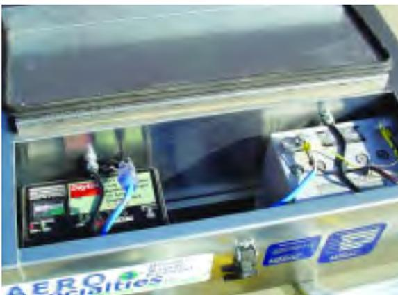
Battery & charger in insulated, sealed compartment
